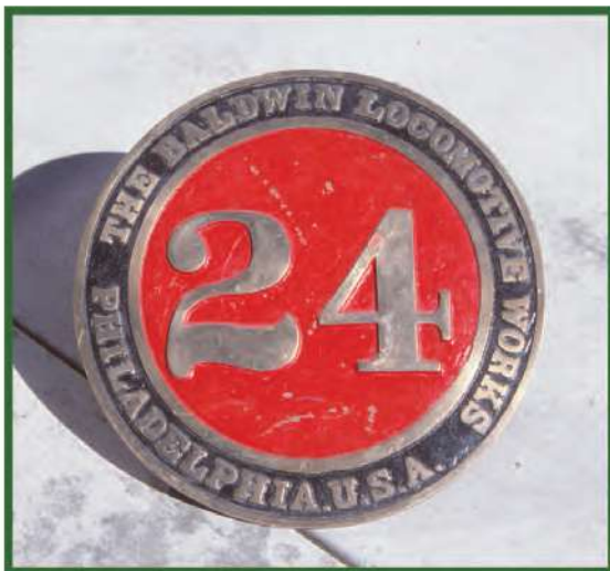
REPLICA BUILDER'S PLATE MADE USING THE ORIGINAL PLATE FROM 2-8-0 No. 24 AS A PATTERN.
