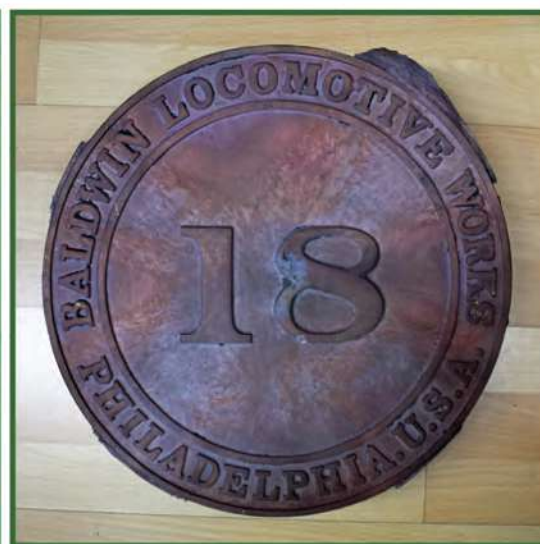
REPLICA BUILDER'S PLATE MADE USING THE ORIGINAL PLATE FROM 2-8-0 No. 18 AS A PATTERN. THE CASTING IS STILL IN ITS RAW FORM.
