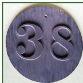
WOODEN PATTERN TO CHANGE THE ORIGINAL NUMBER PLATE FROM WEYERHAEUSER No. 4 TO SIERRA No. 38.
