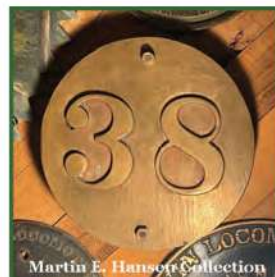
BRASS CASTING MADE FROM PATTERN FOR 2-6-6-2 No. 38's NUMBER.
